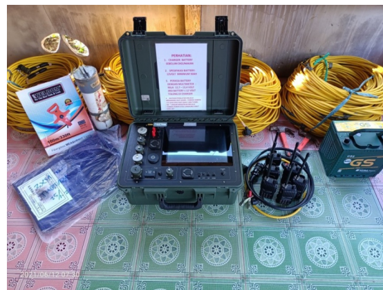
Figure 4. The multichannel geoelectrical instrument MAE .
