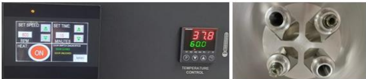
Gambar 2 Pengaturan Alat Koehler Heated Oil Centrifuge
