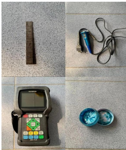
Gambar 3. Ultrasonic Thickness Gauge, Blok Kalibrasi, Couplant, dan Probe
